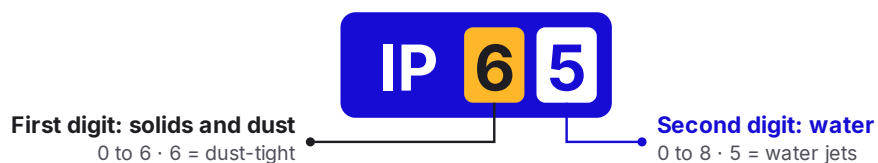
Figure 6.14 How to read the IP rating
